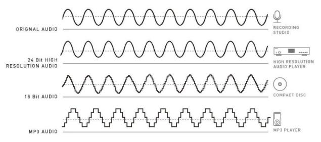
Increasing the bit depth, along with increasing the sample rate, creates more total points to reconstruct the analog wave.
