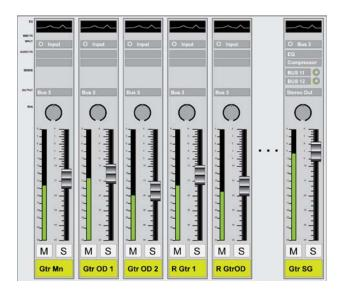
After the levels have been adjusted in each track of the subgroup, the levels and any insert effects on the bus track are collectively controlled on the bus track. To make things more manageable, you can hide the subgroup members leaving only the subgroup track.
